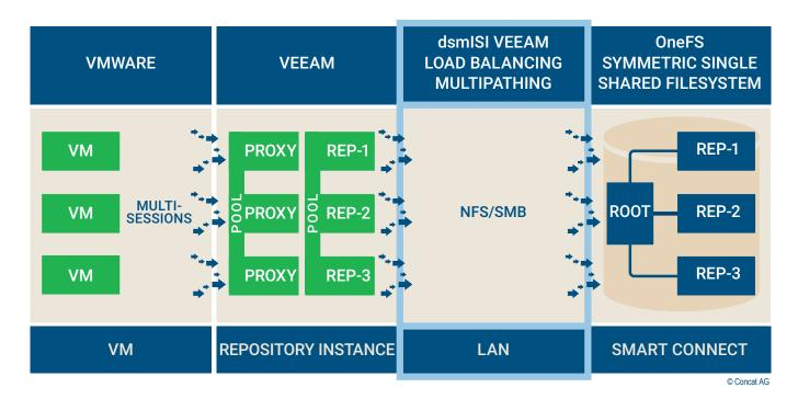
dsmISI Veeam implements dynamic multipathing by automatically spreading reads and writes symmetrically across all available network paths and Isilon nodes, guaranteeing maximum throughput for any attached Veeam repository server.
